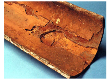
Fig.1 Example internal corrosion (Ref.1)
